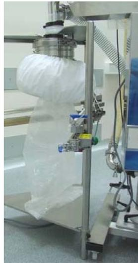
8. Continuous liner Tablet Collector
