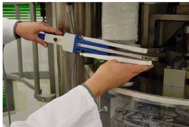
4. Heat-sealing and cutting of lay-flat tubing
